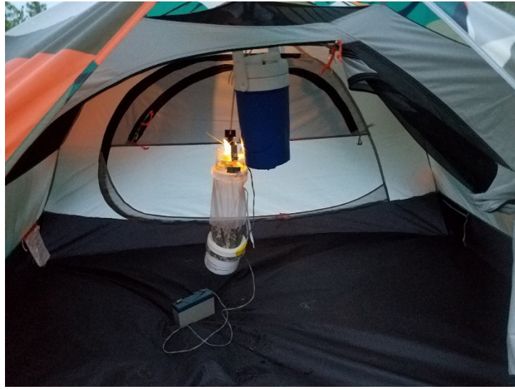
FIGURE 3. PLACEMENT OF CDC LIGHT TRAP (WITH COLLECTION CONTAINER) BAITED WITH DRY ICE PELLETS IN 1.9-L IGLOO COOLER SUSPENDED INSIDE EACH OF THE TWO-PERSON TENTS DURING THIS STUDY.
